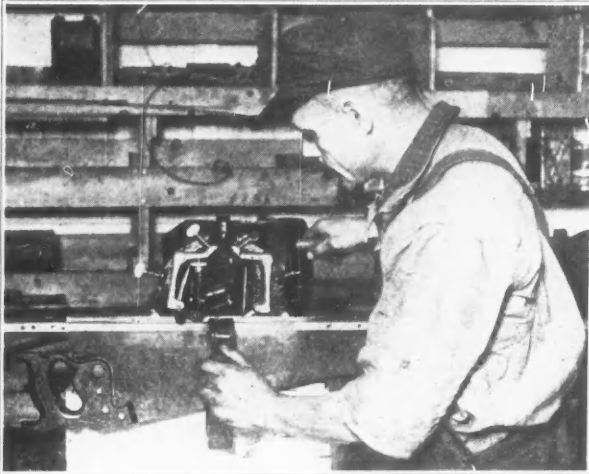
The Automatic Saw Filer Can Be Used for Filing Any Type of Saw With Quick and Accurate Results.
