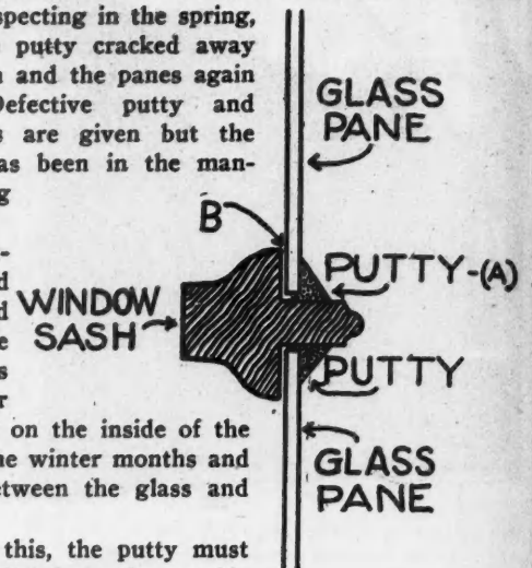
Putty or Paint at the Point "B" Will Exclude the Moisture Which Causes Loosened Panes.
