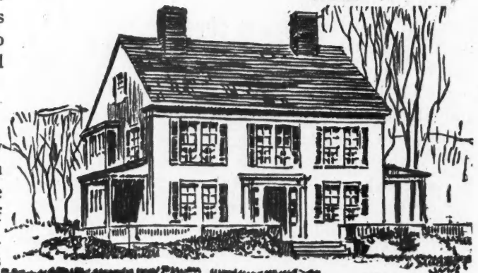
View Showing New Pitched Roof and Side Porches in Alteration One. Floor Plans Are Unchanged.
