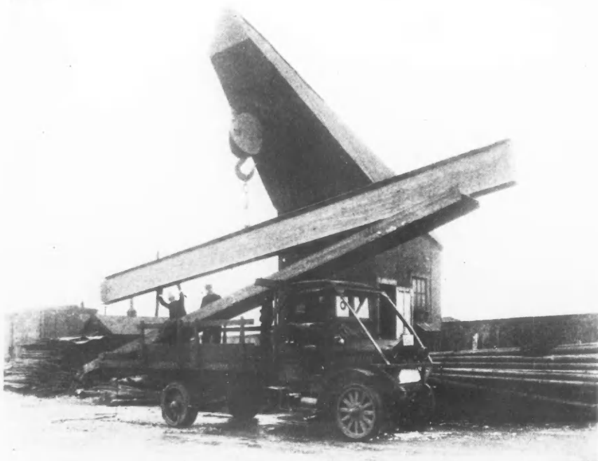
When the Boston Structural Steel Co., Cambridge, Mass., Started to Haul Their Steel Beams and Trusses in Trucks They Found the Stock Body Would Not Fit, so They Built a Special Body on Their Five-Ton "Selden" Such as Is Shown Here and Now Carry Great Steel Beams Without Any Trouble.
