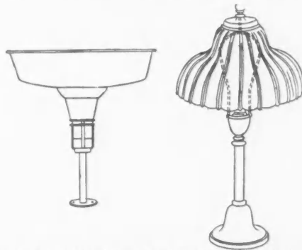
A Simple Means of Obtaining Semi-Indirect Effects from a Direct Lighting Luminaire and the Efficient R. L. M. Standard Dome Reflector for Lighting the Basement and Garage. The Porcelain Enamel Resists Attacks of Moisture.
