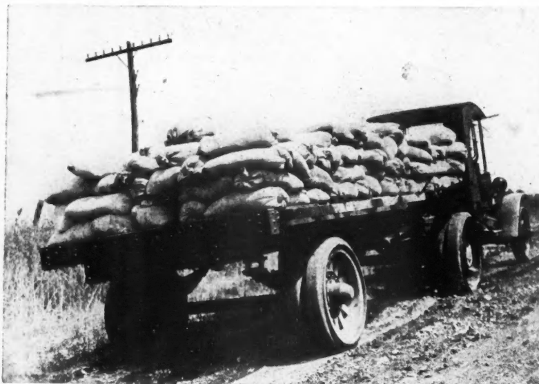
Ten-Ton "Highway Trailer" Negotiating a 14 Per Cent Grade with 25,000 Pounds of Cement, or Just 2½ Tons Overload. It Seems to Carry Its Burden Very Easily. The Unit Is Being Pulled by a Seven-Ton "Sterling" Truck.
