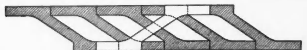
Showing How Each Unit Cross Blinds Five Others and Breaks Joints on Both Sides of All.
