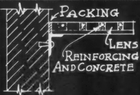
METHOD OF SUPPORTING SIDEWALK LIGHTS AT WALL OF BUILDING
