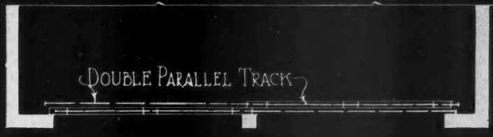
PAIR OF SLIDING DOORS USING DOUBLE TRACK. THREE OR FOUR DOORS MAY BE HUNG IN THIS MANNER.
