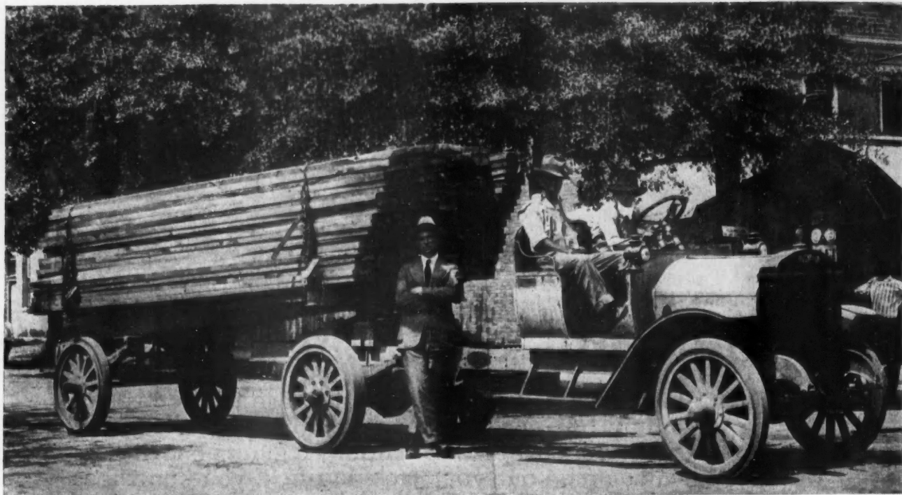
Two-Ton "Indiana" Truck with Semi-Trailer That Has Been Working for the Sipsy River Lumber Co., Aliceville, Ala. Their Specialty Is Long Hauls and Prompt Service. They Save Considerable Time Using Trailers to Eliminate Delay at Loading Points. A Loaded Trailer Is Hooked on as Soon as the Empty One Is Detached.
