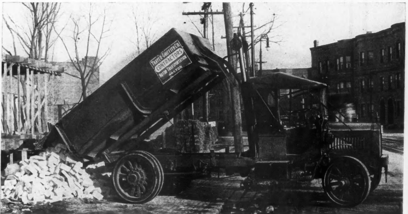
Five-Ton "Packard" Truck Equipped with Hydraulic Hoist for Dumping. It Is Driven Off the Truck Gearset Because of the Heavy Weight to Be Lifted. This Device Will Dump a Load of Gravel in Fifteen to Thirty Seconds. The Truck Can Be Started While the Dump Is Being Lowered.
