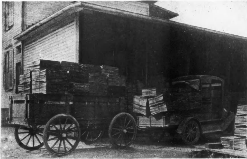
Small Trucks and Trailers Make Efficient Haulage Equipment in the Lumber Yard. Here is a "Miami" Trailer that More than Doubles the Capacity of the Truck to Which It Is Attached.
