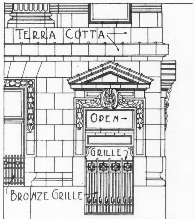
CORNER ENTRANCE DETAIL
