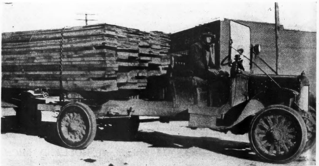
Thru Mud and Over Heavy Roads this "Republic" Truck and Semi-Trailer Transport Big Loads of Lumber to the Building Job. Note the Mud on the Wheels and Chassis. That Gives an Idea of What this Truck Has Hauled the Large Quantity of Lumber Thru.
