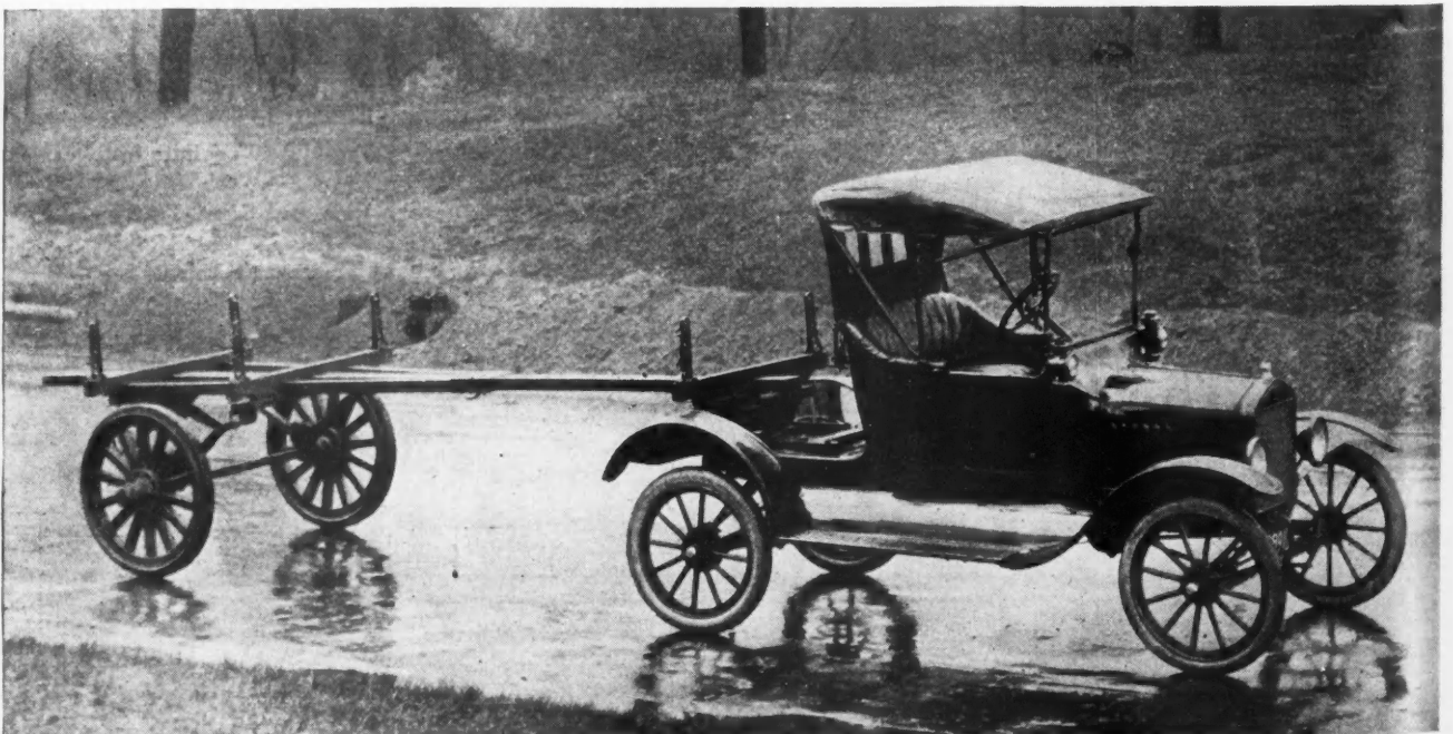
One of the Many One-and-One-Half-Ton "Martin" Semi-Trailers Used by the Edward Hines Lumber Co., Chicago. The Extension Reach Permits this Trailer to Be Used in Hauling Lumber of Various Lengths.
