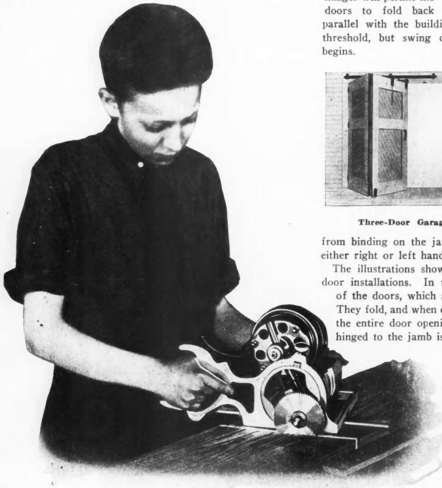
A Circular Saw, Driven by Electricity and Guided by Hand. Its Operation Is so Simple that a Boy Can Use It. Guides in the Bench May Be Set at an Angle, so that Any Cut Desired Can Be Obtained.
