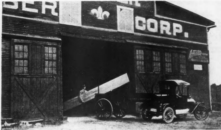
A "Martin" Semi-Trailer, Attached to a Small Runabout, Does the Delivering for the Fletcher Lumber Co. Note How Flexible this Equipment Is Thru the Method of Attaching the Trailer to the Automobile.
