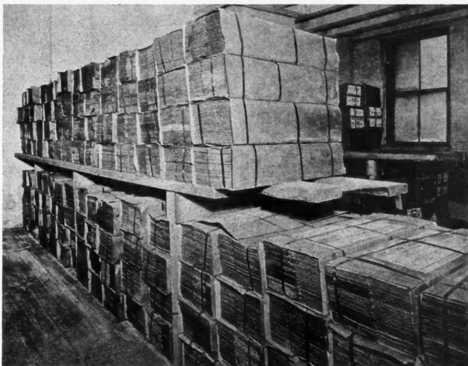
Figure B. Asphalt Strip Shingles Stack in a Boston Warehouse, Using the Tier Method Described.
