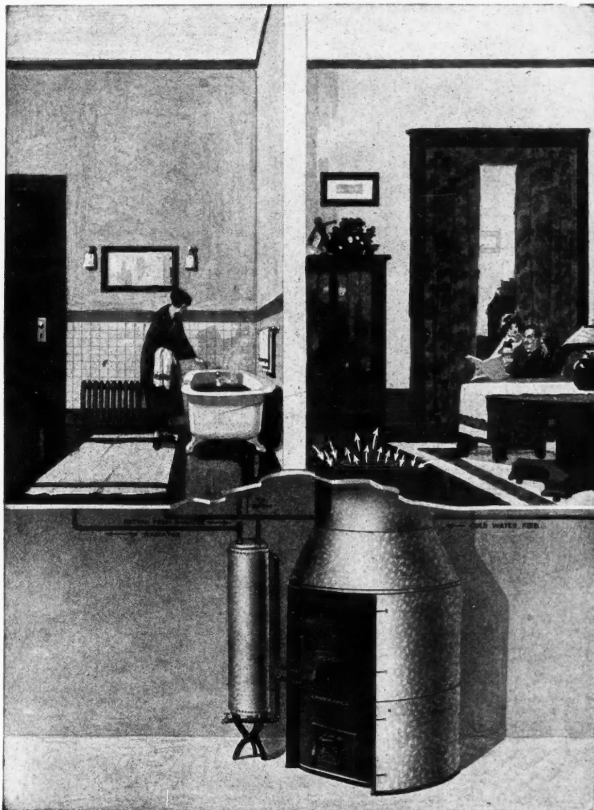
Hot Water Radiator Heats Bathroom or Other Detached Room.
