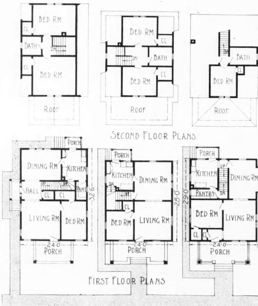
First and Second Floor Plans of Street of Three Industrial Homes Illustrated Above.
