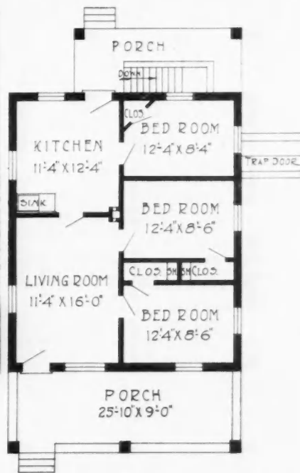
Plan of Tile Cottage. Size, 25 Feet 10 Inches by 30 Feet 6 Inches, Exclusive of Porches.
