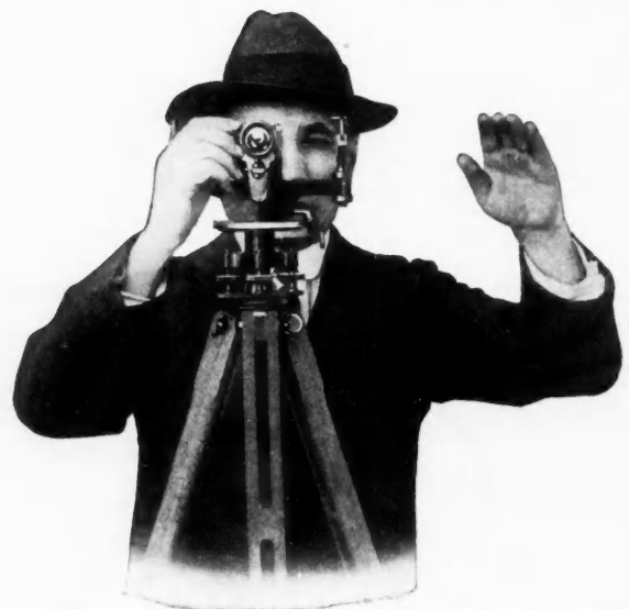
A Convertible Level is Coming to Be Considered as a Necessity in the Equipment of the Modern Building Contractor.
