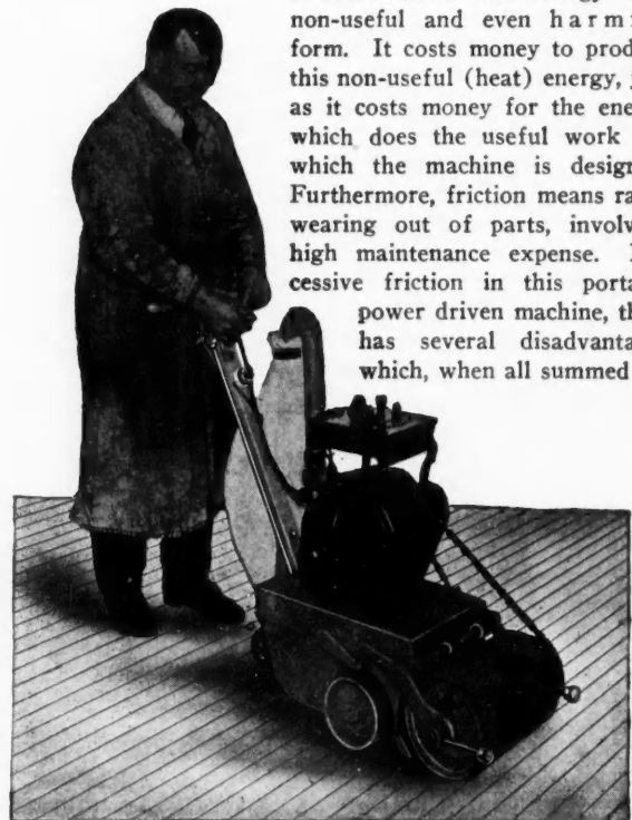
A Modern Floor Surfacer Which is Equipped with Ball Bearings of the Type Shown on the Following Page.
