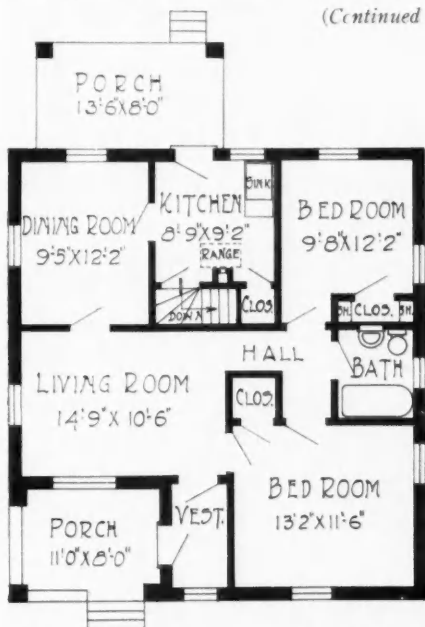
Plan of Small Tile House. Size, 30 Feet by 32 Feet 5 Inches, Exclusive of Rear Porch.
