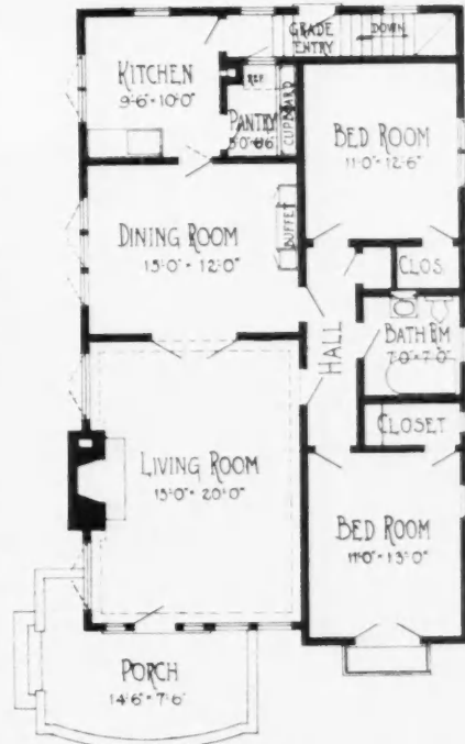
Floor Plan of Bungalow, Size 27 feet 6 inches by 44 feet.
