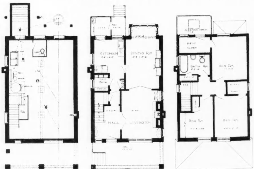
Floor Plans of Typical Narrow Lot, Two-Story City House Built of Brick.
