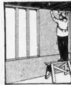
Nail top center first with fine wire brads
