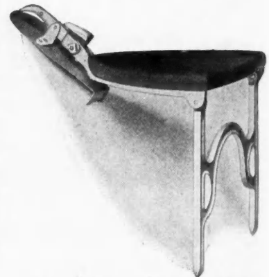
Chair in Position as on Roof—Gripping Device Ready to Clamp onto Shingle End.
