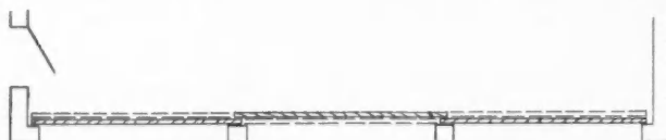
Fig. 23. Three Doors on Two Parallel Tracks
