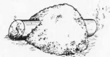
Fig. 2. Culvert Pipe with Fire in One End, for Heating Aggregates
