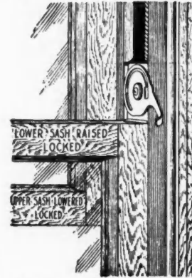
Ventilating Sash Lock Holds Sash Secure in any Position
