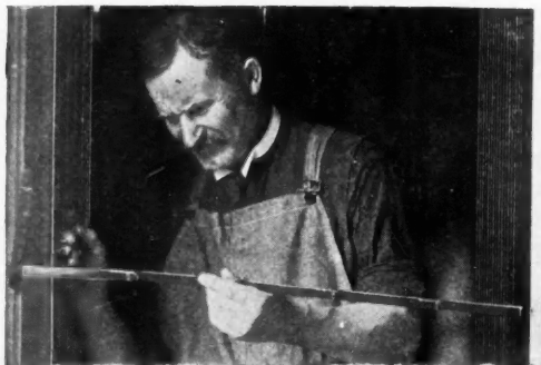
This illustration shows the ordinary carpenters' rule in use for measuring inside window trim. No inside measurement can be taken with the old style rules.
