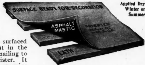
Shows Construction of Bishopric Wall Board
