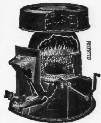
The Underfeed Furnace with casing removed, cut away to show how coal is forced under fire, which burns on top.
