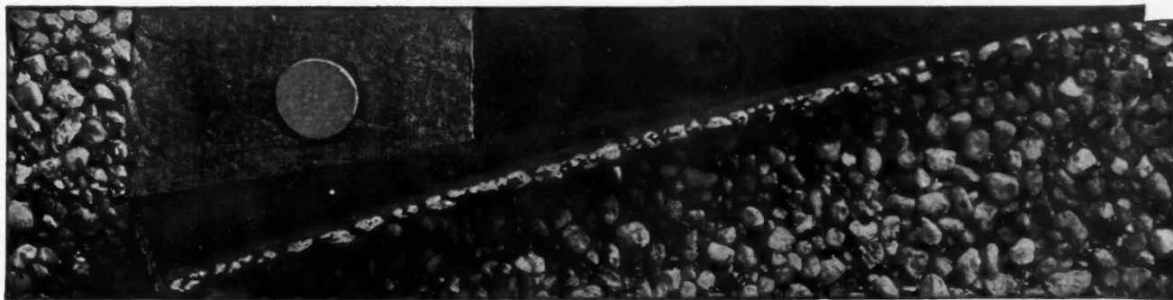
Wide Welded Joint for Heavy Mineral Surfaced Roofing. The Two Uncoated Surfaces are Cemented Together With Hot Asphalt, Covering the Nailing Edge and Forming a Water-tight Joint
