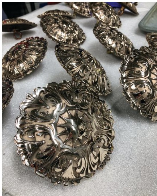
ABOVE, FROM LEFT To create the two-tone design, brass "filigrees" are jet-cut then polished and mounted to the inner sides of the chandelier rings; intricate rosettes are not single pieces but assembled from multiple lost-wax castings; the G-40 LED lamps give a traditional globe appearance without the bulk of incandescent hardware, such as fitters.
