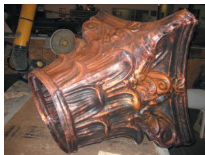
Heather & Little fabricated this copper capital.
