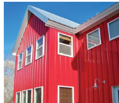
This SL Nail Strip, from Bridger Steel , is a concealed fastener panel with a built-in nail flange for easy installation - no clips required. It is offered with 1-in. and 1 1/2-in. rib heights. Click on No. 2082
