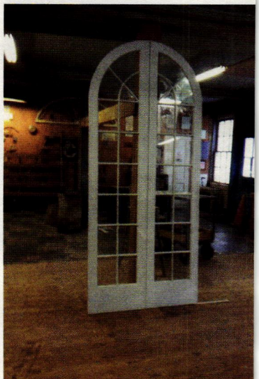
These large double elliptical arch-top French doors were built by Illingworth Millwork .
