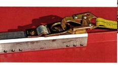
The SSRA1 from Fall Protection Distributors consists of a solid aluminum body with 12 stainless steel set screws and a swivel d-ring; it is designed for use on standing-seam metal roofing.
