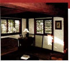
Vinyl-framed, glass interior storm windows from Innerglass were installed in this room and contain concealed stainless-steel spring sytems to seal tightly, and eliminate drafts, condensation and noise problems.
