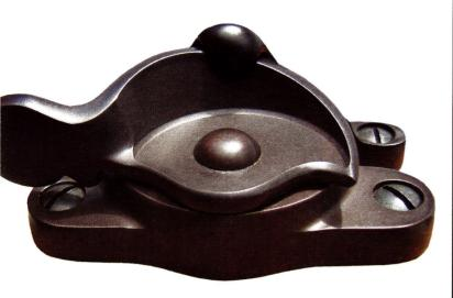
The model LKF18 sash lock from Phelps Company is hot-forged from solid brass and CNC machined; it features a double stainless-steel spring mechanism for smooth operation.
