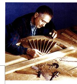
This artisan from Timberlane is putting together a solid kiln-dried western red ædar shutter using mortise-and-tenon joinery.
