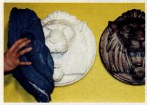
MasterMold, a non-toxic polyurethane paste from Abatron, is used to reproduce both large and small flexible molds.
