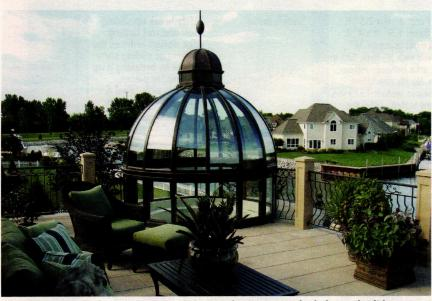
This dome skylight from **Solar Innovations** utilizes 1-in. insulted glass and solid copper and bronze panels.
