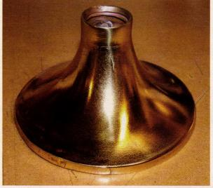
Aurora carefully removed the corrosion, matched missing metal pieces, then brushed and refinished each fixture. Photos: Aurora Lampworks
