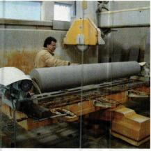
A column shaft of Indiana limestone is being turned on a lathe operated by a craftsperson in the 20,000-sq.ft. studios of Traditional Cut Stone, Ltd.
