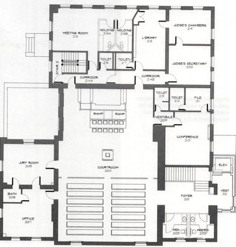
The Federal-style building was expanded to include a story-wing with a second-floor courtroom (above, right) and a three-story jail. The new elevator addition is situated between the chimney of the original building and the exterior corner adjacent to the early addition.
