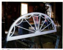
Jim Illingworth Millwork manufactured this attic halfround window sash with spiraled web using singlepane glass and true-divided lites.
