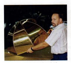
This bronze cupola was custom-designed and manufactured by C&J Metal Products and is available in copper, lead-coated copper and galvanized steel.
