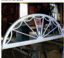
Jim Illingworth Millwork manufactured this attic halfround window sash with spiraled web using single-pane glass and true divided lites.
