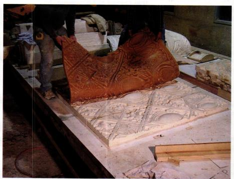
Rubber molds for the GFRC were cast from the assembled plaster masters.
