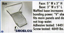
Face: 5" W x 3" H Base: 3" W x 5" L Waffled base increases bonding power. "V" shape fits more panels and does not trap water. Adhesive tested: 1449 lbs.
