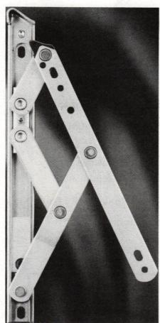
A 4-bar friction hinge from BRONZE CRAFT supports projected vents from 10-1/2 to 79 in. H. and weights from 82-220 lbs. It also supports casement vents 10-1/2 to 33 in. and weights from 84-103 lbs. Other features: Stainless steel slide mechanism, concealed nylon wear strip, and a built-in, nonremovable variable stop to comply with child safety guidelines. Write in No. 838
