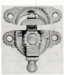
One of BALL & BALL's many styles of window hardware, this Victorian cast-iron sash lock (#V150-225) measures 2-1/2 in. W. and requires a 7/8 in. width on the upper sash for mounting. Write in No. 293
