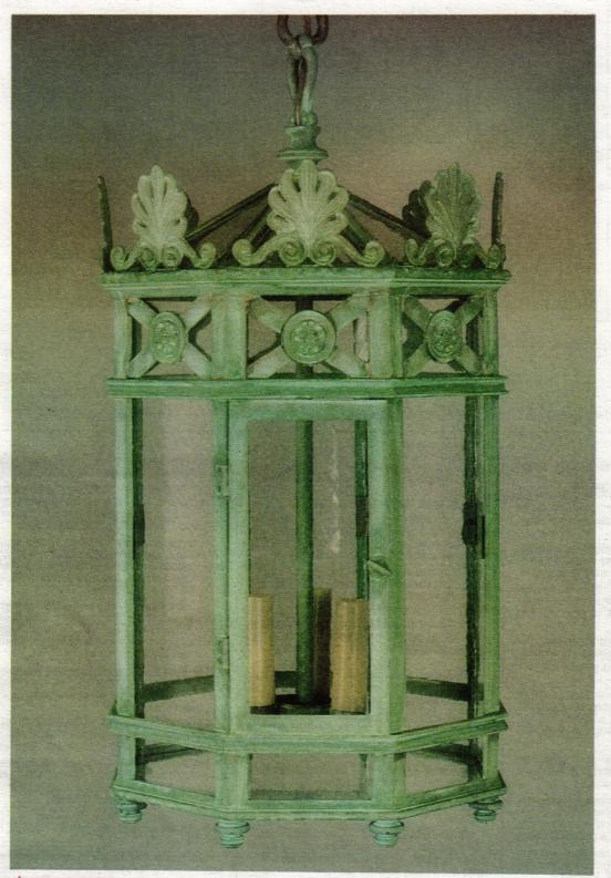
▲ Fixture # 1004. 12" wide x 25" tall. Cast brass octagonal hanging fixture suitable for exterior use. This Fixture is fitted with hand blown sheet glass. Relamping access is fitted through a hinged pane. A wall mounted version is also available.
