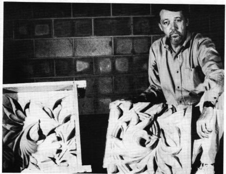
Stan Townsend, of SYNAIR CORP., poses with his mold, made from a twocomponent system, and a model, made from a two-component casting resin. Write in No. 725
