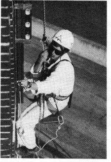
Harry Littell, of the structural inspection and testing service VERTICAL ACCESS, investigates a brick veneer failure. Write in No. 476
