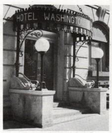
L.M.C. CORP. designed and fabricated the entrance marquee of the Washing-ton Hotel, in NYC. It features a glass roof and wrought-iron brackets with gilded monogram.
