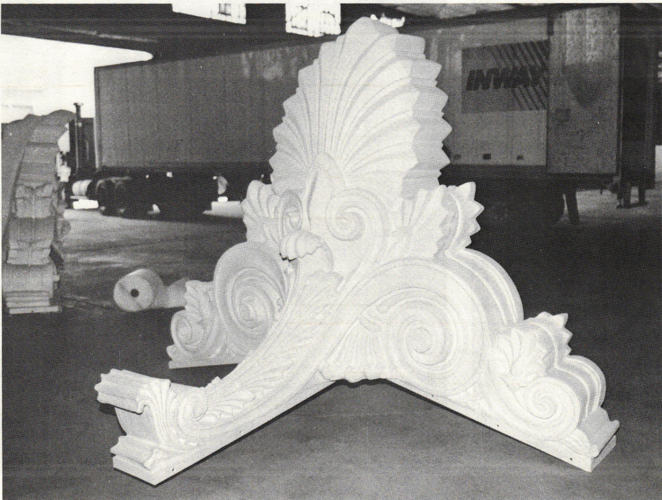
Brackets (with styrofoam cores) were precast in architectural concrete by ARCHICAST as part of the reconstruction of an Italianate cornice.
