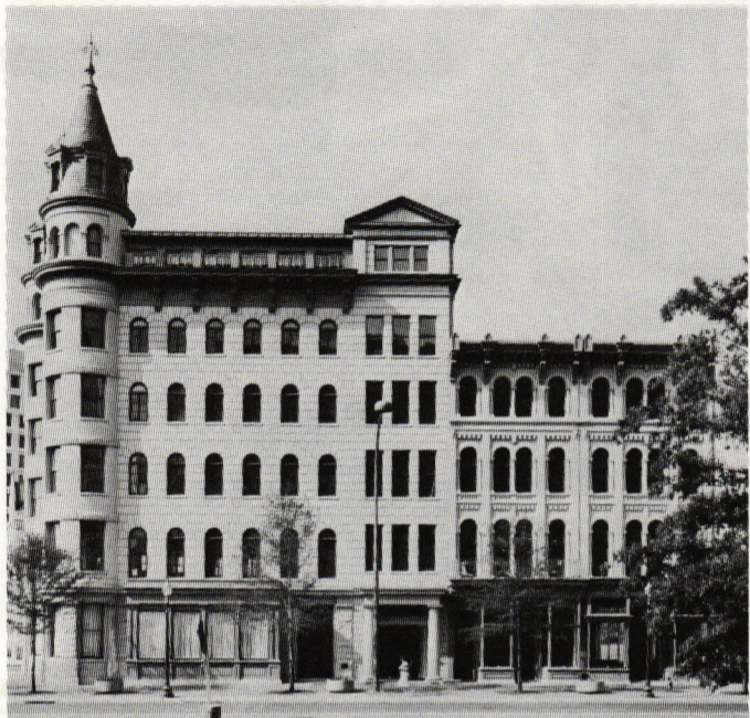
Our favorite example: Two historic buildings in Washington, D.C., skillfully joined with a tall, narrow infill section that houses mechanical equipment, elevators, and fire stairs. Design Architect: Hartman-Cox Architects. Architect: Geier Renfrow Brown (Phase I), Leo A. Daly (Phase II). Preservation Architect: John Milner Associates.
