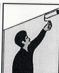
12. Apply 2nd coat of saturant (include seam)
