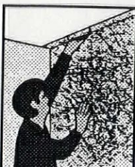
4. Trim excess mat where wall meets ceiling.
