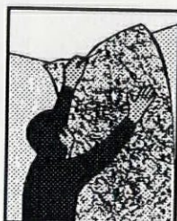
3. Apply fiberglass mat to wet surface.
