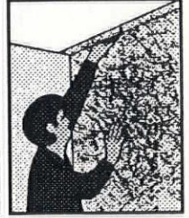
4. Trim excess mat where wall meets ceiling.
