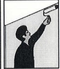
12. Apply 2nd coat of saturant (include seam)
