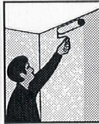
2. Apply saturant to area to be covered.
