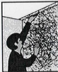
4. Trim excess mat where wall meets ceiling.
