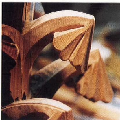
A close-up of the finished detail. Note that the glue line is straight, thin, and almost invisible.
