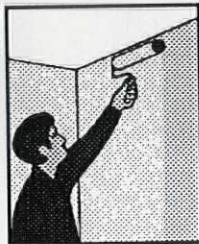
2. Apply saturant to area to be covered.
