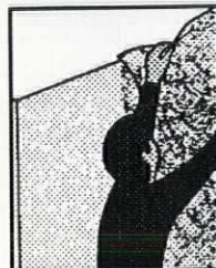
9. Apply mat to 2nd area, overlapping by 1".
