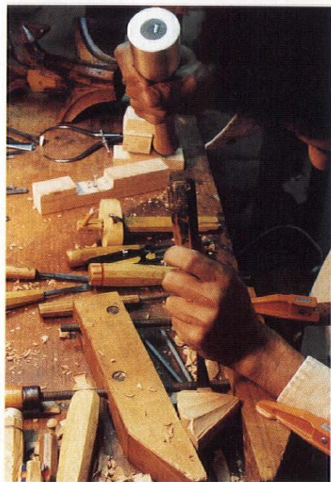
The mallet comes into play when extra force and control is needed. Even with the mallet, however, the wrist is still anchored to the work.
