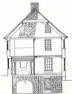
Note the massive timber framing and basement entrance in this cross-section plan of Fort Bowman.
