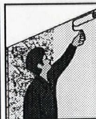
8. Apply 1st coat of saturant to adjacent area.
