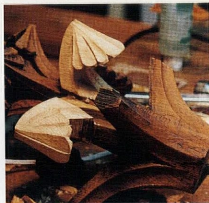
Broken surfaces must be planed flat before gluing. Note that the new necks are still oversized.
