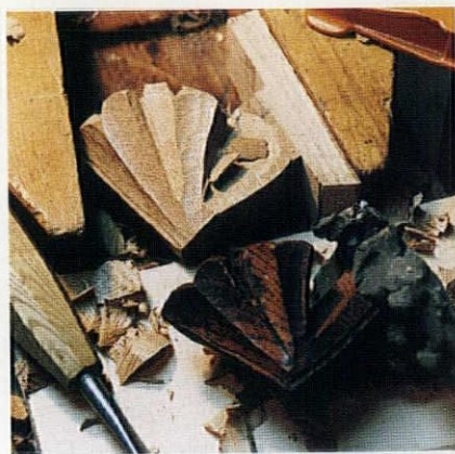
With the sample as a model, Calvo next roughs out the form using a variety of chisels. Clamps hold the wood.
