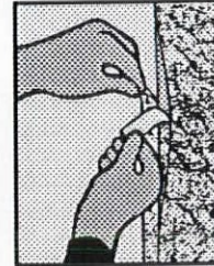
11. Remove mat strips on both sides of cut.
