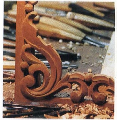
This bracket—an example of pierced carving—will be attached to some larger woodwork in the room.
