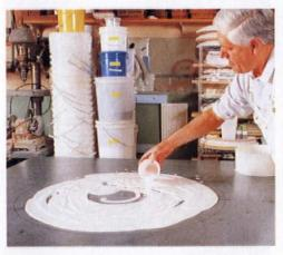
When ready, mix up plain gypsum plaster (plaster of paris) and apply it onto the board in a ring the size of the medallion.
