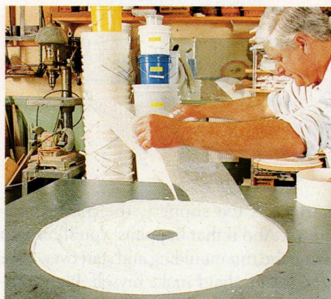
To strengthen the disk, add sheet fiberglass or erosion control burlap cut to shape, and then pour on more plaster.
