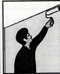
12. Apply 2nd coat of saturant (include seam)
