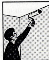
7. Apply second coat of saturant to wet mat.
