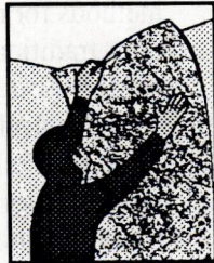
3. Apply fiberglass mat to wet surface.
