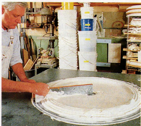
Attach the pivoting arm and spin it through the plaster. Where needed, feed additional plaster ahead of the revolving blade.
