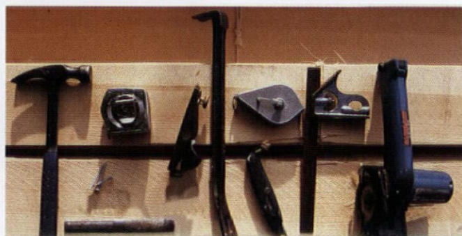
Clapboarding Tools: claw hammer (with slightly rounded face), tape measure, low-angle block plane (sharp), wood rasp, pry bar, chalk line, utility knife, square, cordless trim saw (or fine-toothed crosscut hand saw).
