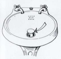
Silicone makes a new seal under a drain-plug lip.
