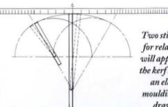
Two sticks set up for related radii will approximate the kerf spacing of an elliptical moulding (top of drawing).
