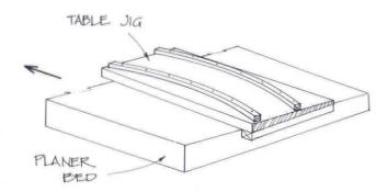
To set up for production planing, make a jig angled to the bevel of the siding and adapted to mount to the thickness planer bed.
