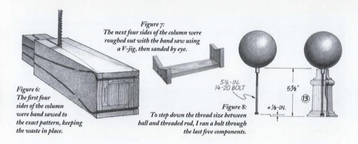
flat to accomodate the T-nut. The next step was to centerbore the whole column — a ½" hole from the top and a %" hole (for a little slop factor) from the bottom — using a bit extender to get all the way through. I center-bored the upper column section with a ½" bit, enlarging the top hole to accept the ball fitting and chiseling the bottom hole square to recess the bolt head.
