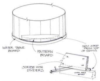
Making a pattern board: Place the board on the wall so the ends touch the base leaving a gap at center (exaggerated for clarity). Then scribe the gap measurement along the bottom to trace a curve (inset).
