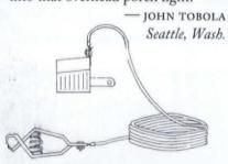
Hardware stores supply the adapter plug, alligator clip, and insulated wire needed to make a ground jumper.
