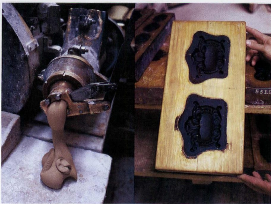
Left: Compo manufacture begins by extruding the raw mixture from a blending machine. Right: Molds are carved from maple blocks with black asphaltum cores and might be used for decades.
