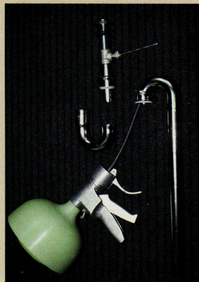
Left: When snaking a lavatory drain, begin at the outlet after first removing the stopper (which may block the snake). Right: If the snake binds at the trap, disassemble it or enter at a cleanout closer to the blockage.
