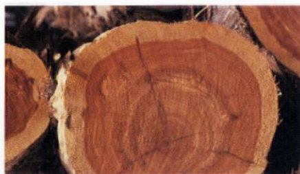
This cedar log butt highlights the division between sapwood (the light-colored outer ring) and heartwood (the inner, reddish bulk of the trunk).
