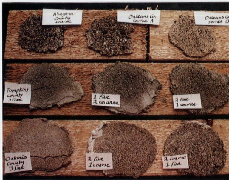
Left: Test samples of lime mortar made from a variety of local sand grades and combined in different proportions provide a
