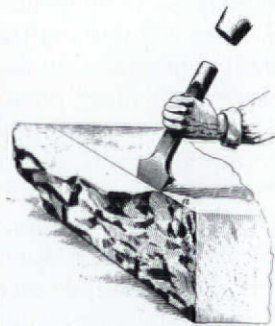
For most operations, chisels should be applied at an angle to the stone face, not perpendicular to it.
