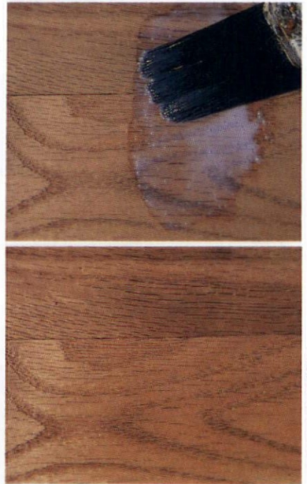
Some new water-based finishes brush on milky (top), but dry clear (above).
