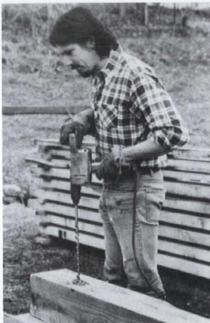
A 1/2-inch drill is a heavy-duty tool that requires using two bands at all times. (Most large bits need its power and 1/2-inch-capacity chuck.)
