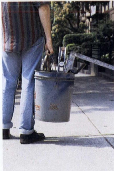
An empty joint-compound bucket is light, low cost, and a popular container for heavy items such as masonry tools.
