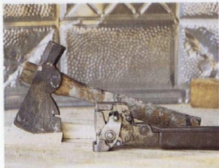
The "business ends" of a carpenter's hatchet and a staple hammer.
