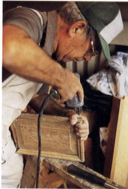
\frac{1}{4} -inch and \frac{3}{8} -inch drills are band-sized tools and essential for general old-house woodworking and repairs.
