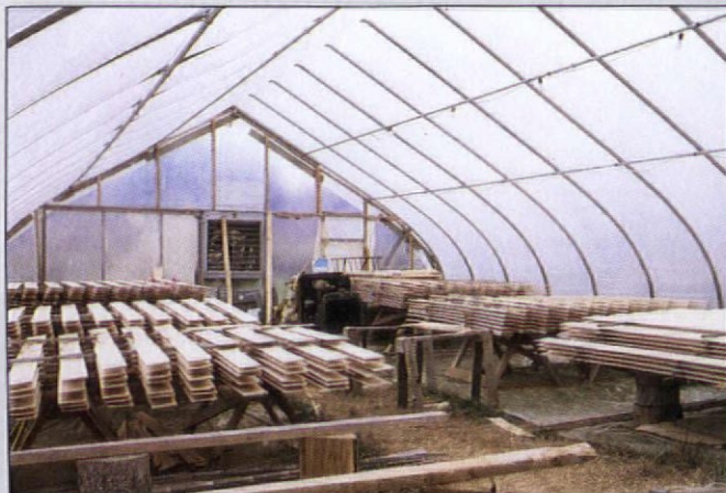
After sawing, clapboards are air dried (rather than kiln dried) to retain the natural resins that give the wood its longevity. A Donnell saying is "Cook your food — not your wood (and not too much)."
