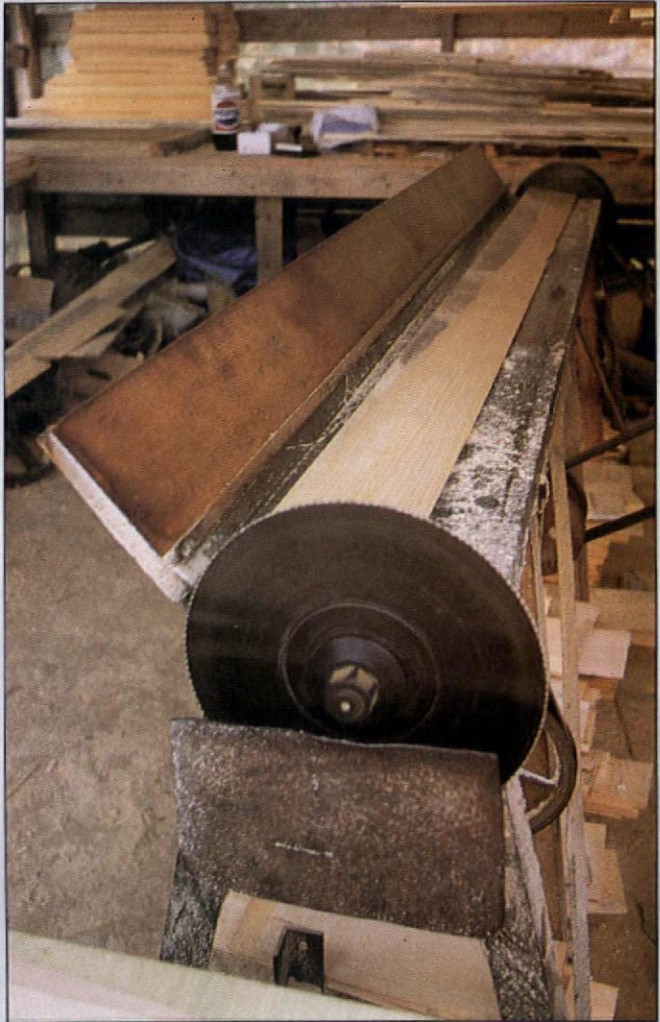
End trimming and grading are the last steps before the clapboards are packaged for shipment.
