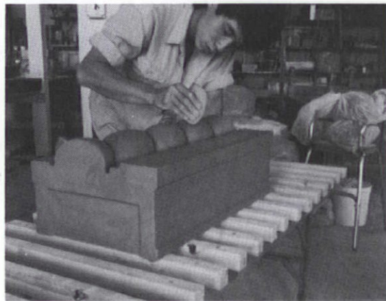
Terra cotta being manufactured. Left: Worker pressing clay into mould. Right: Trimming imperfections in the casting.
