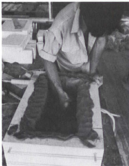
Terra cotta being manufactured. Left: Worker pressing clay into mould. Right: Trimming imperfections in the casting.
