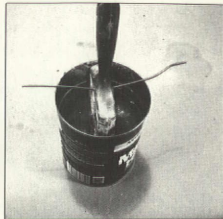
When you leave a neglected brush soaking in solvent, keep it suspended on a wire.
